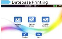
① Can print variable text, QR code and barcode, realizingone object with one code (variable marking).
